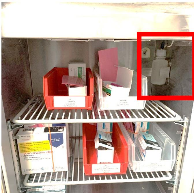
DDL probe placed in dedicated probe location of a pharmaceutical grade unit.
