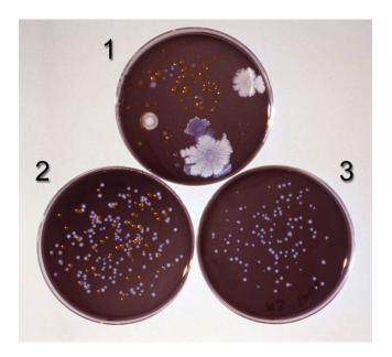
This image shows test plates of environmental (water) samples for Legionella using BCYE agar (plate 1) and BCYE agar and with antimicrobial supplementation (plates 2 and 3), with Legionella colonies most clearly isolated on plate 3. Even with specialized media, Legionella can be difficult to isolate with recommended culture methods due to overgrowth of other bacteria. CDC's Laboratory Guidance also describes using amino acids cysteine and glycine to select for Legionella growth.
